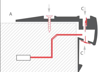
4. Snap in the cover (E) and connect the LED strip to the power supply.
